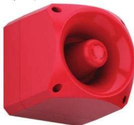
**Siren - Nexus 105/110/120:** Connections on base made during the initial phase, for faster and more reliable installation. In addition, the head is fixed by quarter-turn fasteners that allow a faster, more precise and resistant installation for the compression of the sealing in the open. With IP66, it can be installed almost anywhere. 64 tones, 3 alarm stages. Model 105dB, V=10-60VCC, I= 8-40mA, Model 110dB, V=10-60VCC, I=10-50mA and Model 120dB, V=10-60VCC, I=120-550mA.
