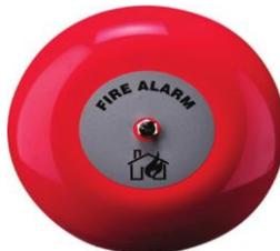
The Fire Bell is a motorized hood designed for fire alarm applications. Its low current consumption and universally recognizable alarm sound makes it an ideal choice for many alarm systems. Designed for easy installation, it features a robust steel gong. Audibility at 1m: max 95dB (A), V:19-28VDC, I:20mA
