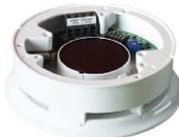
**Base with Siren:** It has a low profile, its main application is for installation together with the patented smoke and heat detectors and provide both detection and alarm at the same point, which reduces wiring and installation costs. With the optional cover it can be used as an individual siren, for indoor use. Available in white and cream colors. Audibility at 1m: up to 95dB (A), Voltage: 17 - 60 VDC, Current (depending on pitch): 2 - 7 mA
